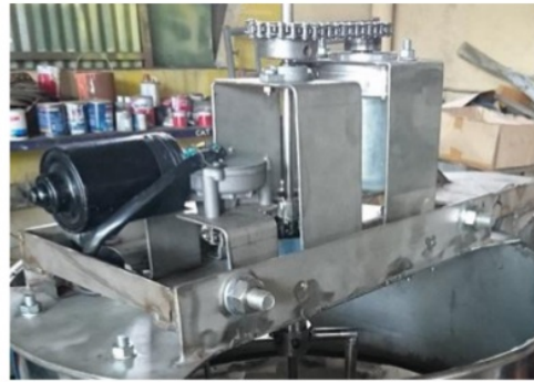
Figure 6. The Transmission of Automatic Flouring Gauge Machine
