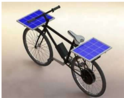
Figure 3. Design of an electric bicycle using solar panels
