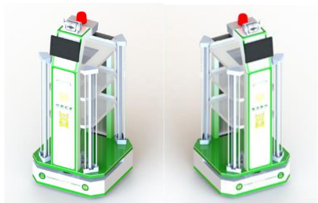
Figure 5. design of paramedic assistant robot 3.0
