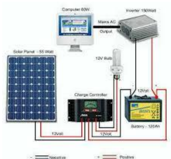
Figure 2. Model of solar PV power generation
