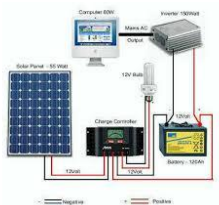
Figure 2. Model of solar PV power generation
