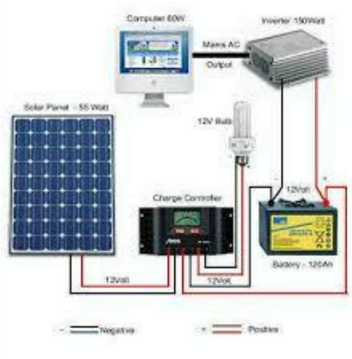
Figure 2. Model of solar PV power generation
