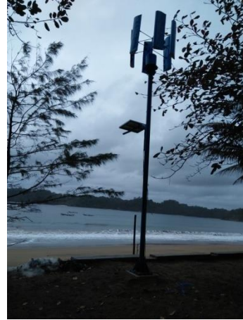
b) Turbin angin Darrieus NACA airfoil 6 blade
