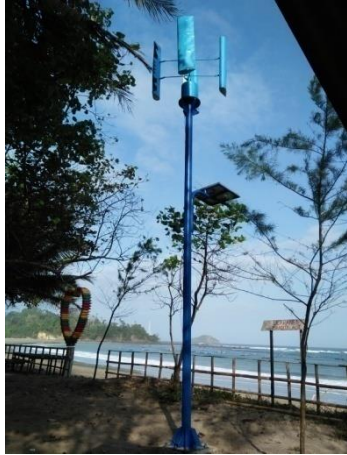
a) Turbin angin Darrieus NACA airfoil 4 blade
