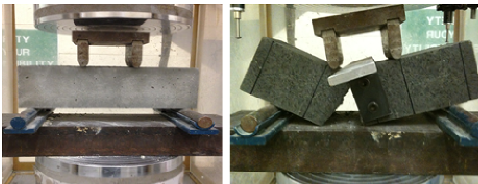
Fig. 1. The apparatus for flexure test of concrete by third-point loading method (ASTM C78-02)
