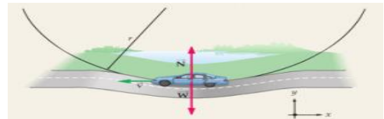
Figure 7: A car crosses the road on a decreasing radius with a radius of 65.0 m depth (Source: Zitzewitz, et al. 2005)
